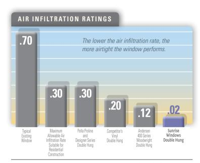
With a constant 25 mile per hour wind, this test shows how many cubic feet of air infiltrates through each square foot of the window each minute. Results are from Pella Product Guide Specification 2008, and Andersen 2009 Performance Standards. Sunrise Casement AAMA Certified 2010. Sunrise Double Hung results from April 2016 testing.
