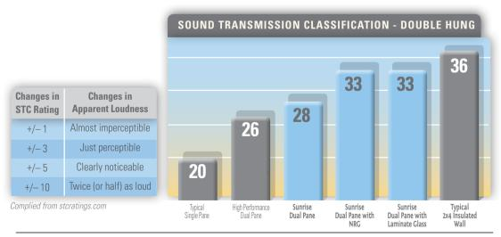
Our windows are tested and rated to ASTM E(90) for Sound Transmission (test sizes per ASTM E1425). STC ratings will vary by product type. The higher the rating value the greater the sound reduction.
