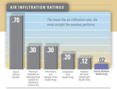
With a constant 25 mile per hour wind, this test shows how many cubic feet of air infiltrates through each square foot of the window each minute. Results are from Pella Product Guide Specification 2008, and Andersen 2009 Performance Standards. Sunrise Double Hung results from April 2016 testing.
