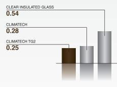
\*Performance based on whole window values of an 0501 Double-Hung Window.
